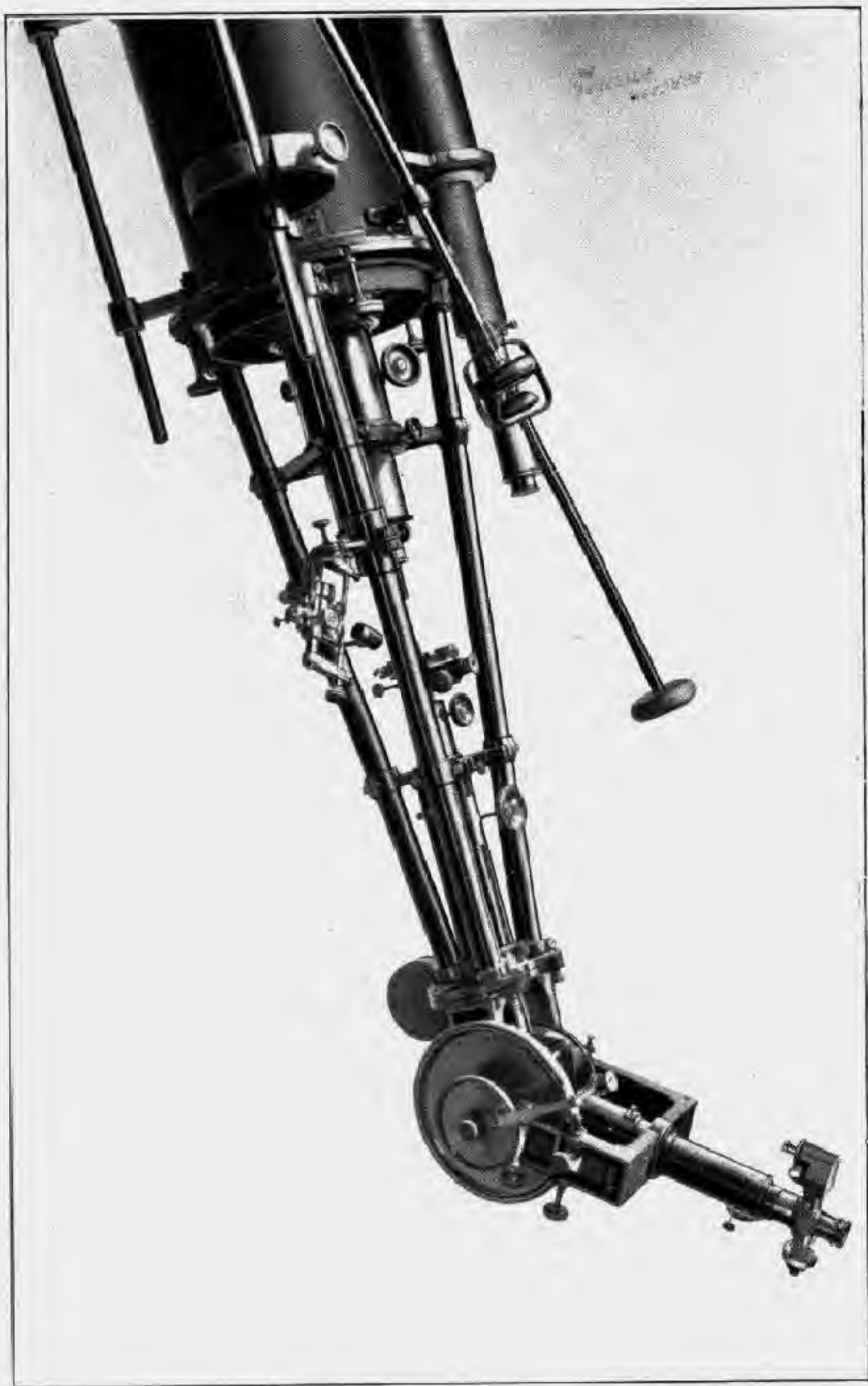
Spectroscope and Spectrograph. Made for Allegheny, Yerkes and United States Naval Observatories. Engraving shows adaptation for one prism. See page 30.
